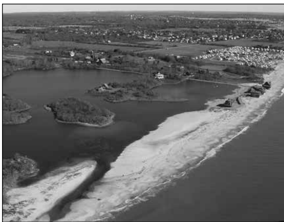
Figure 3. Aerial photo by S. Paton of US Fish and Wildlife Service taken several days after Sandy, showing overwashed sand on the coastal barrier in front of Cards Pond in South Kingstown. Note the location of the Browning Cottages at the right edge of the photo.
