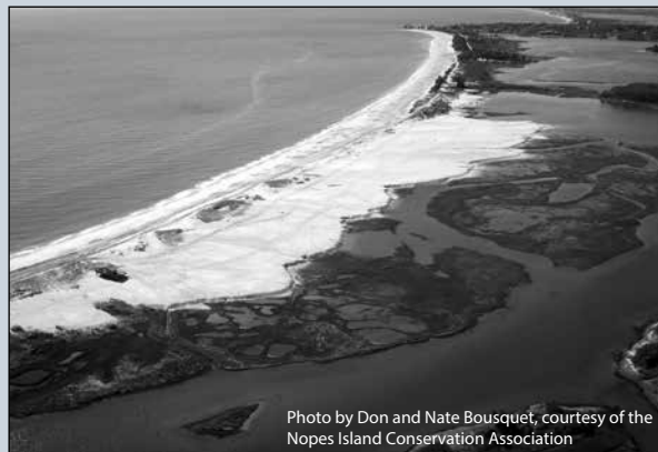
The storm surge from Sandy caused significant overwash of sand onto the coastal barriers which separate the salt ponds from the ocean. The two middle photos show the Quonochontaug Barrier before and after the storm. Note the location of the "slip slope", or pondward boundary of the overwash, revealed at lower left of each photo. The top of the slip-slop indicates the high-water level in the pond--this is where the storm surge dropped sand when it receded (above right). Also note that Japanese black pines planted on the western end of the barrier (top of photos) prevented sand from washing over, creating a "reflective" rather than "dissipative" dune front. Sand also washed over the Green Hill Barrier (below, left) and East Matunuck beach in front of Pt. Judith Pond but did not reach the ponds. Surprisingly, most of the major overwash on the Misquamicut Barrier (below, right) also did not appear to reach Windward Pond.
