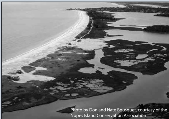
The storm surge from Sandy caused significant overwash of sand onto the coastal barriers which separate the salt ponds from the ocean. The two middle photos show the Quonochontaug Barrier before and after the storm. Note the location of the "slip slope", or pondward boundary of the overwash, revealed at lower left of each photo. The top of the slip-slop indicates the high-water level in the pond--this is where the storm surge dropped sand when it receded (above right). Also note that Japanese black pines planted on the western end of the barrier (top of photos) prevented sand from washing over, creating a "reflective" rather than "dissipative" dune front. Sand also washed over the Green Hill Barrier (below, left) and East Matunuck beach in front of Pt. Judith Pond but did not reach the ponds. Surprisingly, most of the major overwash on the Misquamicut Barrier (below, right) also did not appear to reach Windward Pond.
